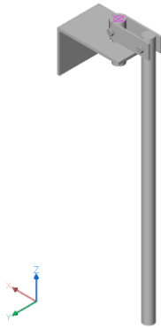
SwtOpSA Switch, Operator, Swing Arm
